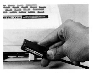
This is how the system should look after you have connected the recorder to the computer. (Back view)
