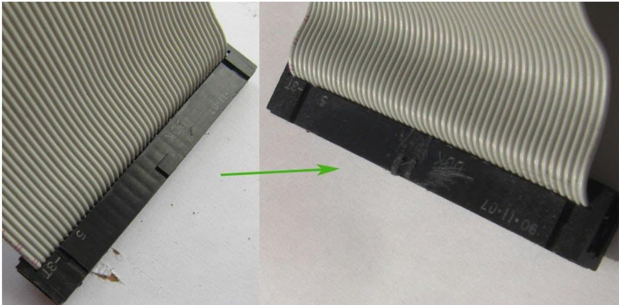
4) Separate each wire on the other end about 1 cm with a cutter and cut all even cables (2, 4, 6, ..., 50) 6 mm with scissors.
