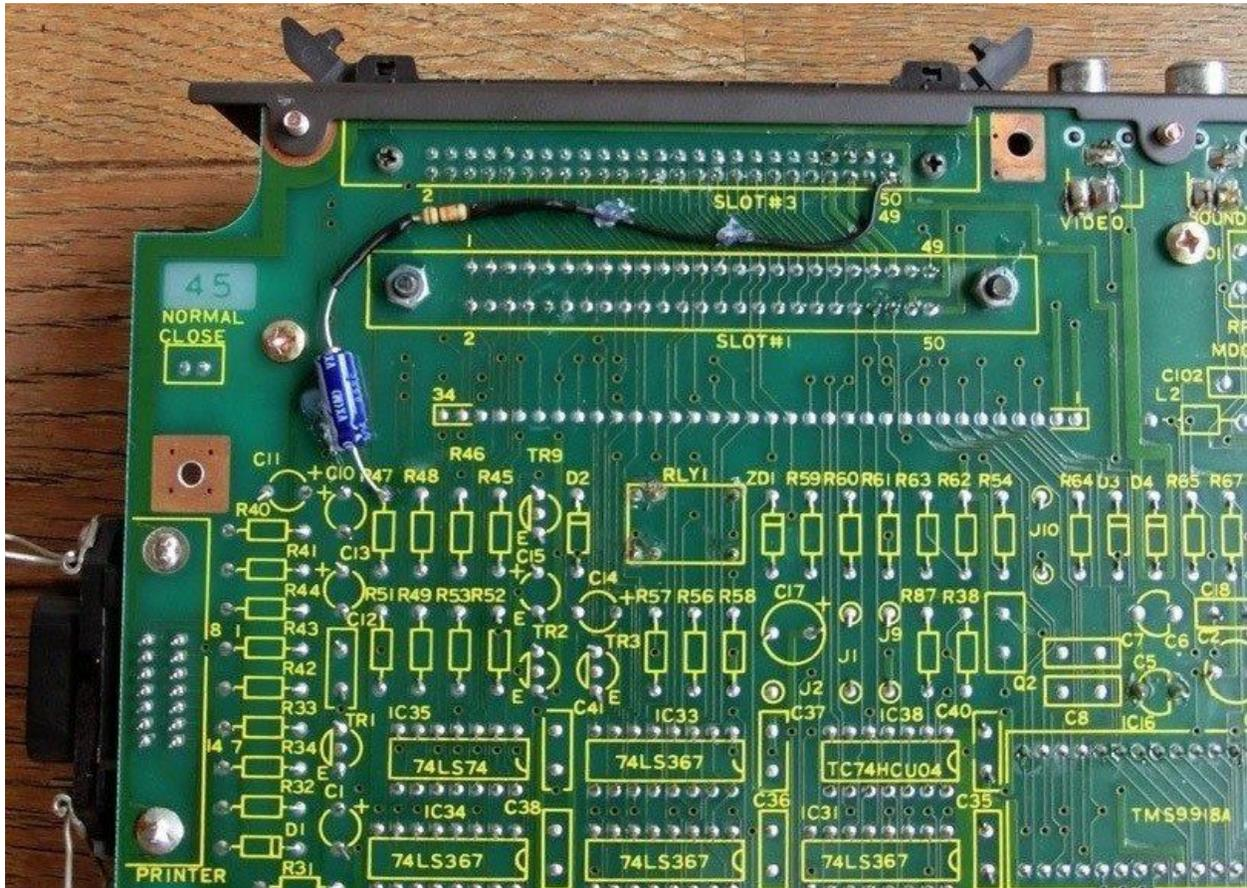
Pin 49 of the SLOT-3 is connected to a 10 K $\Omega$  resistor which is connected to the (-) side of a 10  $\mu$ F capacitor. The (+) side goes to the amplifier. Now the Slot is 100% functional.
