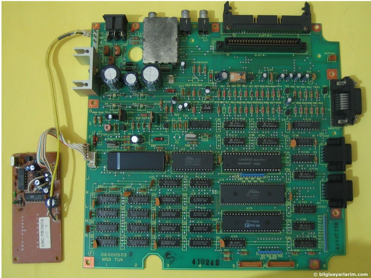
On some computers like the HX10 the **SOUNDIN** (pin 49) seems not connected. You can fix that, find the audio combine inout point of the audio amplifier on the PCB by following the resistor/capacitor line from the cartridge connector to pin 49 on the cartridge slot. A bit complicated without circuit diagram to explain, it is usually a resistor and a capacitor in series. Here is how GDX did it on a HX-10.
