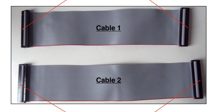
Polarization keys on the opposite sides of the cable
